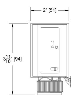
**Engineering Specification:** Zurn four wire zone valve motor. Zone valve motor is a fast acting (10 seconds to open) motorized zone valve actuator. Up to eight valves per 40VA transformer.
