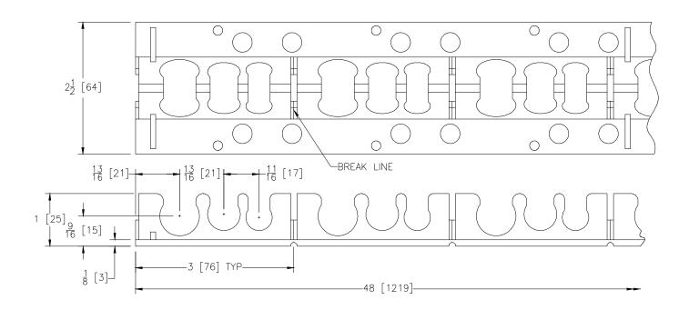
**Engineering Specification:** Zurn Radiant Panel Pipe Track. Track in 4' lengths with minimum 3" spacing. Supports barrier and non-barrier PEX tubing at a constant height with even spacing. Pre-drilled holes allow for easy fastening to a rigid surface. Pipe track holds 3/8", 1/2" and 5/8" tubing.
