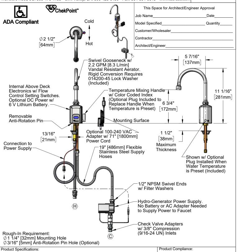
Chrome Plated Brass Above Deck Electronics Faucet, Single Hole Deck Mount, Swivel/Rigid Gooseneck, 2.2 GPM VR Aerator, Point-of-Use Temperature Control, Hydro-Generator Powered, Stainless Steel Flexible Supply Hoses & 3/8" Compression Inlets
