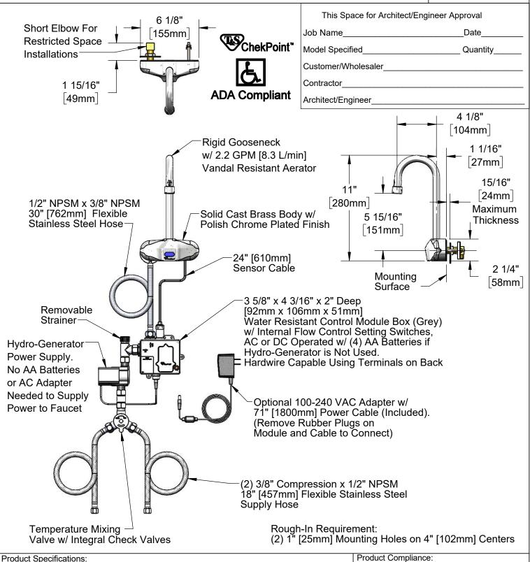
Chrome Plated Brass Electronic Faucet: 4" Wall Mount Rigid Gooseneck w/ 2.2 GPM VR Aerator, AC/DC Control Module w/ Internal Flow Control Setting Switches, Temperature Control Mixing Valve w/ Integral Check Valves, Hydro-Generator & 18" Hot & Cold Supply Stop Flexible Connector Hoses
