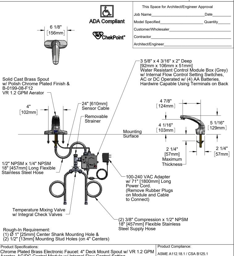
Chrome Plated Brass Electronic Faucet: 4" Deck Mount Spout w/ VR 1.2 GPM Aerator, AC/DC Control Module w/ Internal Flow Control Setting Switches, Temperature Control Mixing Valve w/ Integral Check Valves, 18" Flexible Stainless Steel Supply Hoses
