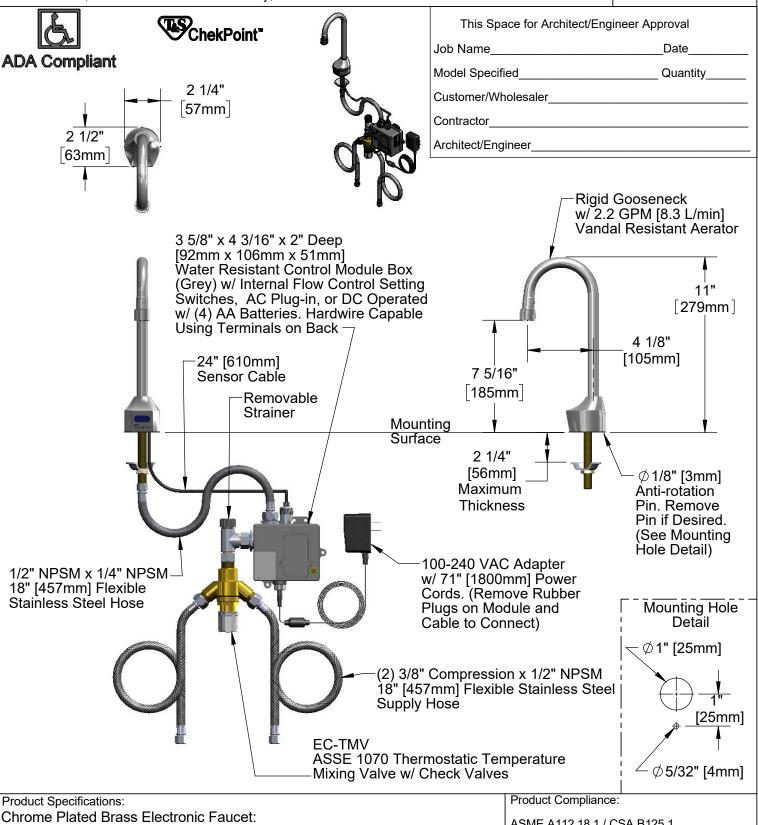
Deck Mt. Rigid Gooseneck w/ VR Aerator, AC/DC Control Module w/ Internal Flow Control Setting Switches, Thermostatic Temperature Control Mixing Valve w/ Check Valves, 18" Hot & Cold Supply Stop Flexible Connector Hoses
