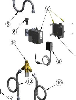
A Maximum of (8) ChekPoint Faucets can be Hardwire Connected and Powered by EC-HARDWIRE ChekPoint Hardwire AĆ Transformer. (Sold Separately)
