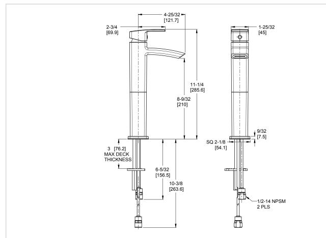
Ø1 Min to Ø1-1/2 Max. Deck Hole Openings
