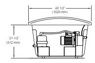
**Installer Note:** Due to the freeform shape of this tub, it is recommended that the tub be on the jobsite before making the final cut out for drop-in installation.
