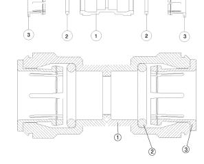
Pictured Mini-Loc Coupling Cutaway view
